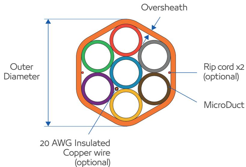
The silicon core-micro ducts can be installed into existing larger sub ducts and can be used to increase the carrying capacity of the duct network. Micro ducts are intended for protection of optical micro cables and are not designed for permanent inner pressure.
