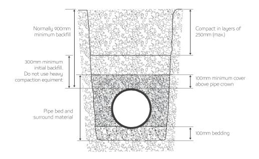
Where a free flowing rounded single size granular material having a maximum particle size of 10mm and very few fines (pea gravel) is used for the pipe surround trench widths may be reduced to only 100mm greater than the pipe diameter.
