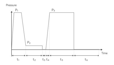
P1: fusion (jointing) pressure (generally 0.15 N/mm<sup>2</sup> + drag pressure)
