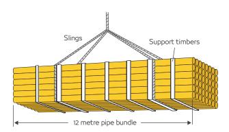
Some deflection or slight bending of pipes and pipe bundles is acceptable when loading or unloading. Standard 6m long bundles may be handled by forklift, provided that the forks themselves are covered in a protective wrapping to minimise the risk of damaging the pipes. Longer lengths should be loaded and unloaded using either a crane with a spreader bar and slings that support the pipes at four points or a specialised a side-loader with a minimum of four supporting forks.
