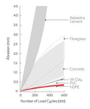
Almona PE80 and PE100 pipes offer outstanding abrasion resistance, making them the first choice for applications where high internal resistance to abrasion is required e.g. for transporting solids in liquid or gaseous forms such as particulate slurry at low velocity and various other industrial effluents. The abrasion rates of our pipe systems increase depend on several factors including:
