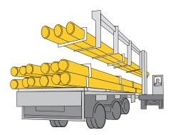
It is the responsibility of the site management to ensure that the site is safe to accept pipe deliveries. The area where the delivery vehicle is to stop shall be safe and the location for storage shall be on firm level ground which is free from sharp and protruding objects and also from any hydrocarbon (typically gasoline and diesel) contamination, which may be absorbed by the pipe wall.
