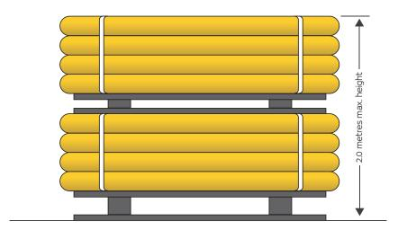
Batches of small diameter pipe coils are sometimes packed on pallets to facilitate storage and transportation. Coils delivered on pallets should remain main secured to the pallet and only be taken off when being prepared for use.
