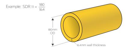
The pressure rating of any homogenious material pipe, regardless of the material, is determined by the SDR and the strength of the material in resisting the hoop stress generated by the internal pressure. The holds true, regarless of the pipe diameter.
