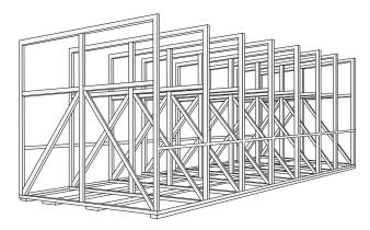
Where large diameter coils are to be transported or stored vertically, they must be secured in purpose-built racking, similar to that shown in the above figure, with protective matting positioned beneath the coil. When transported in such frames the coils must be secured to prevent movement.
