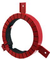
Fire protection collars are recommended to be used when installing the pipes and fittings on walls and ceilings and where active protection measures must be taken. In case of fire or heat, a special fireproof laminate inside the collar begins to expand and creates a protective seal against transmission of fire inside the system.
