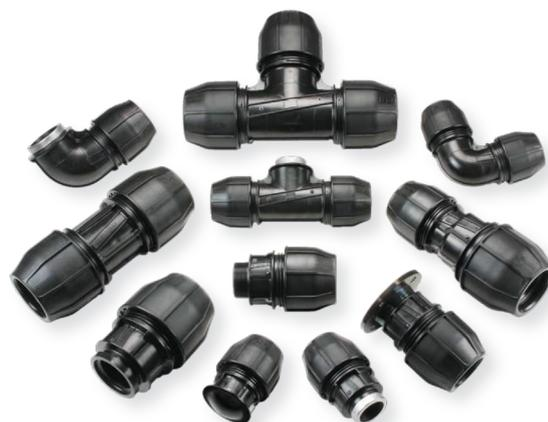
In each case the threaded body and sockets are made of injection moulded polypropylene and fittings used for potable water supply applications should be certified as complying with ISO 17885 – 2015, Plastics piping systems - Mechanical fittings for pressure piping systems – Specifications. It should be noted that there are large quantities on poor quality compression fittings, that do not comply with the standard produced for use in irrigation applications.
